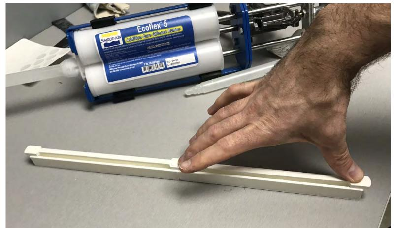
• Fill with a low durometer fast cure silicone, such as Ecoflex 5 (Smooth-On)
